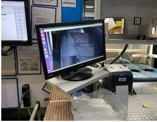
Figure 1: The visual fault detection software and hardware, operator view
